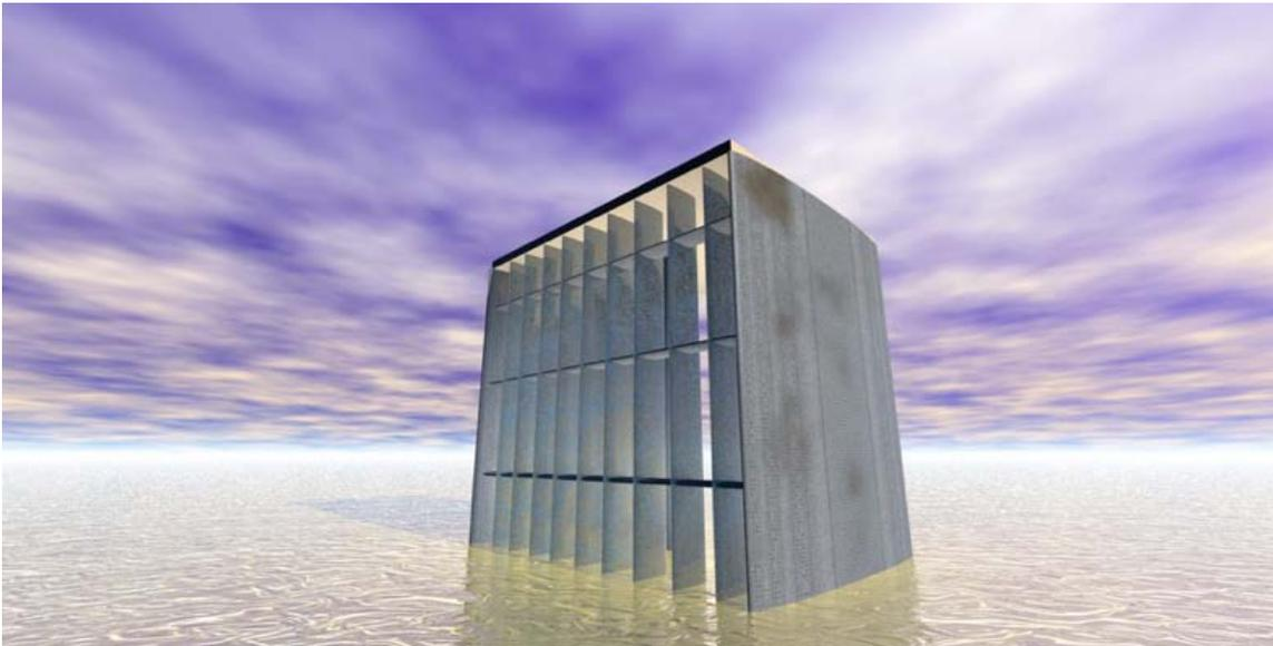
**Figure 4. First Bay Complete.** Each Bay consists of two reinforced end-plinths, a top deck, horizontal louvre supports, full-length sectioned louvres with top-mounted drive motors, and—barely visible—a shaft (pile?) extending from the top deck down to submerged turbine(s). Each Bay is under-lit using light-pipes to convey sun/daylight from the top deck underneath, to prevent shadows of the deck attracting marine life.
