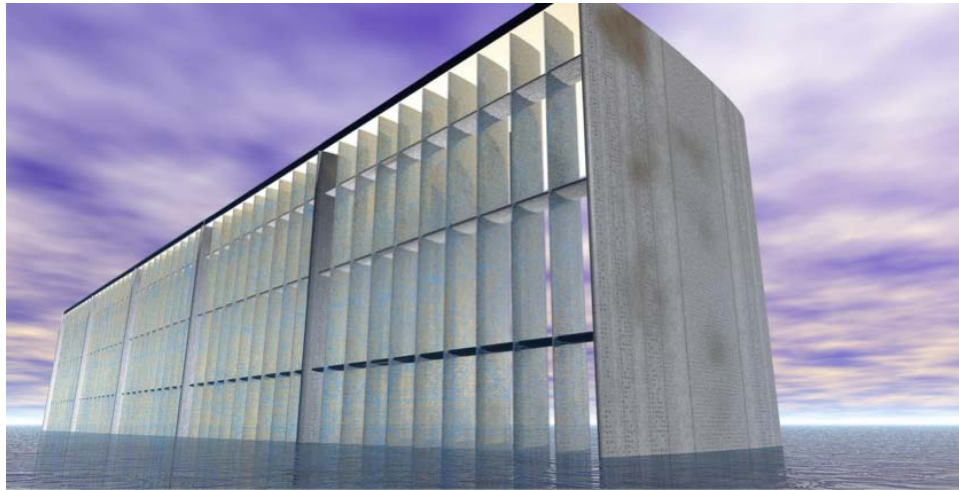
Figure 5. Block of 5 Bays. All bays under-lit, shutters open in streamlined position. The bays will be of a height greater than the highest storm tide, allowing for rising tides and global warming. They will have to be sufficiently robust, too, to resist the impact of Storm Tides that, like a tsunami, may have the potential to arrive as a powerful wave front. This suggests that each bay may be of limited width, as shown, so that there are many reinforced plinths and that louvres are strongly supported and robust. (Shutters may not be vertical louvres as shown: instead, they could be dropped down as needed—c.f. shop window horizontal steel security shutters—leaving the bay open to marine traffic, while the turbines would be deep under the water surface.)
